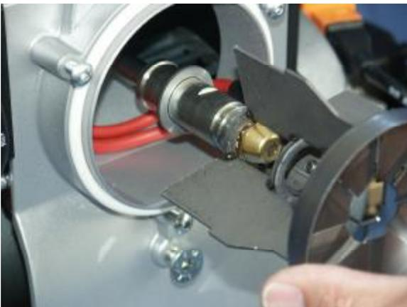
It is important that the nozzle holder is prevented from rotating by use of a second spanner while unscrewing the nozzle
